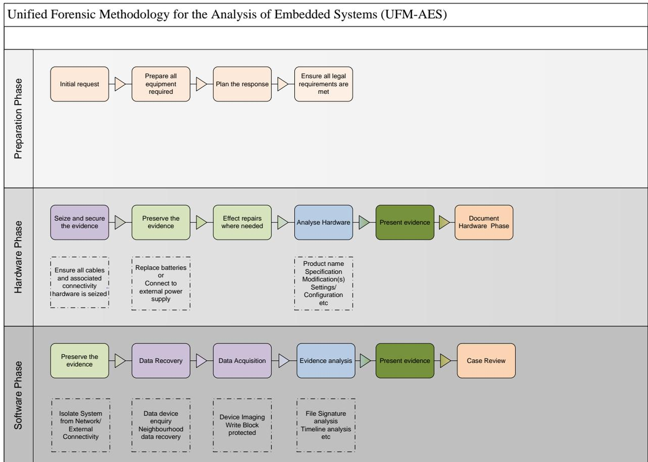
Figure 5 Proposed UFM-AES Methodology for analysing Embedded Systems
