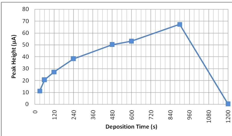
**Figure 4-2: Effect of deposition time on peak height of zinc**
