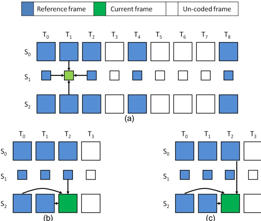
**Figure 5-29** Prediction architectures for a) Hierarchical B-picture, b) Extended architecture based 3D-DMB and c) Proposed prediction architecture
