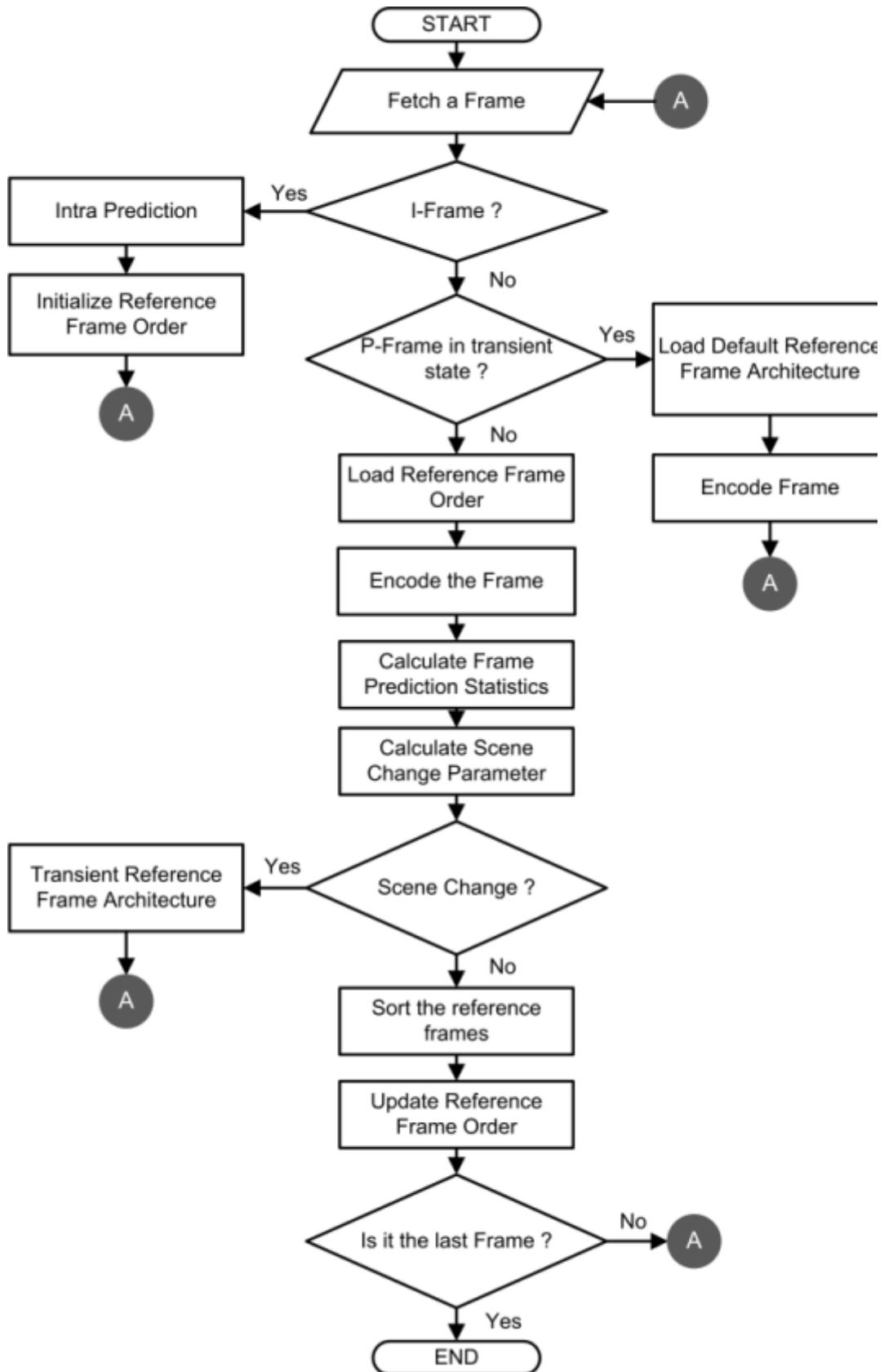
**Figure 4-24** Adaptive reference frame ordering algorithm
