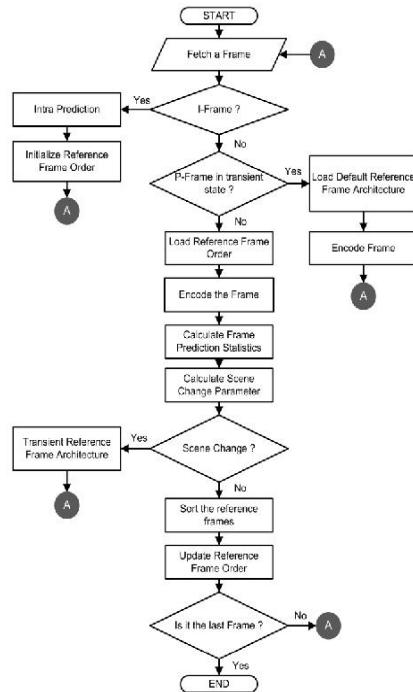
Figure 3 Adaptive Reference Frames Re-ordering Algorithm
