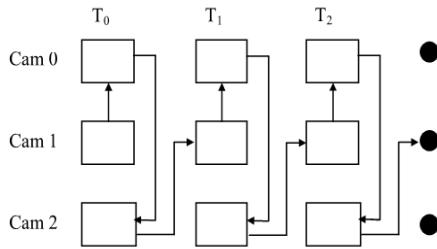
Fig. 2. Interleaving Multi-view videos to generate a single stream video.
