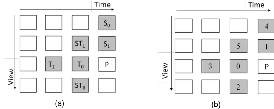
**Figure 5-19** Symmetric multi-view video coding a) RFS and b) RFO
