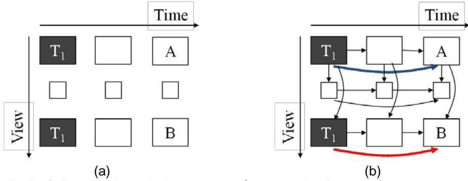
**Figure 5-25** a) Temporal prediction using 2<sup>nd</sup> temporal reference frame source and b) Prediction architecture among three-view video coding
