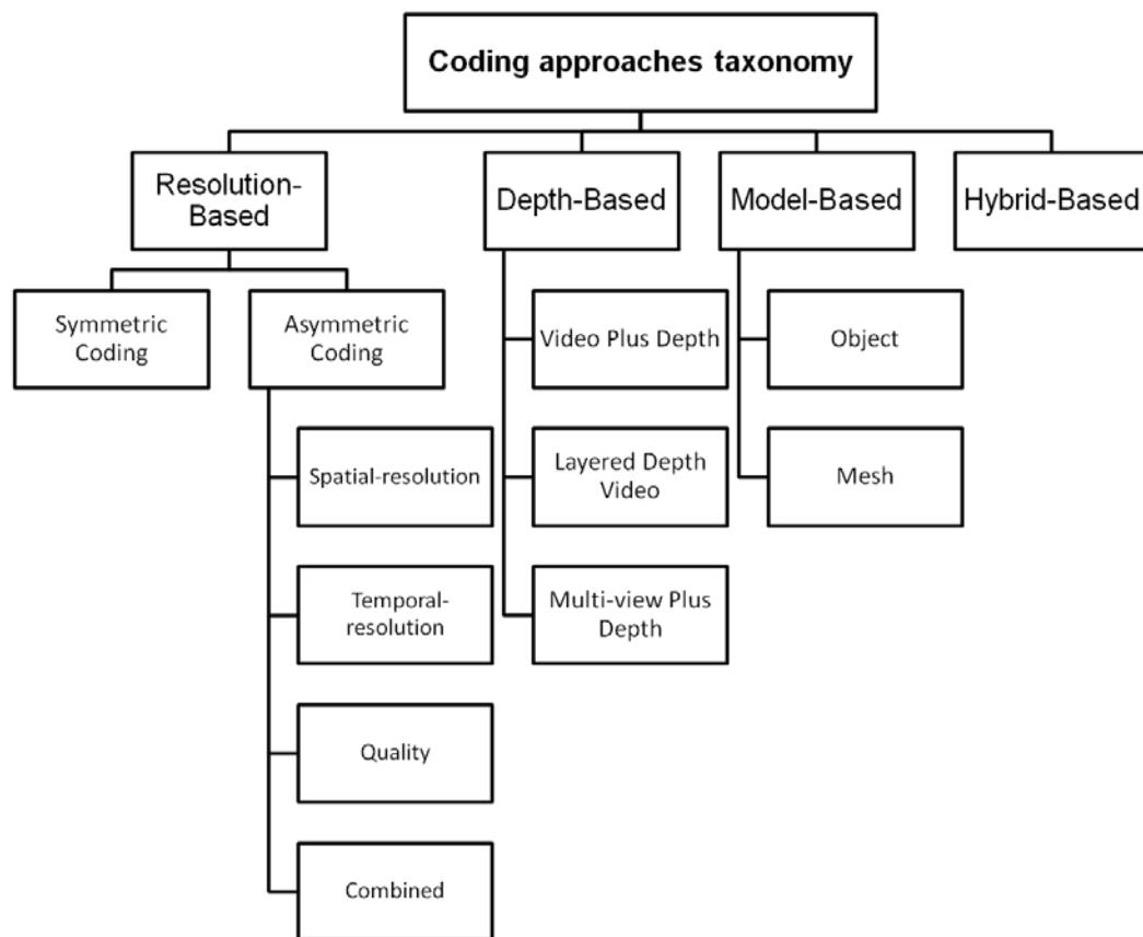
**Figure 3-1** Coding approaches for low bitrate applications
