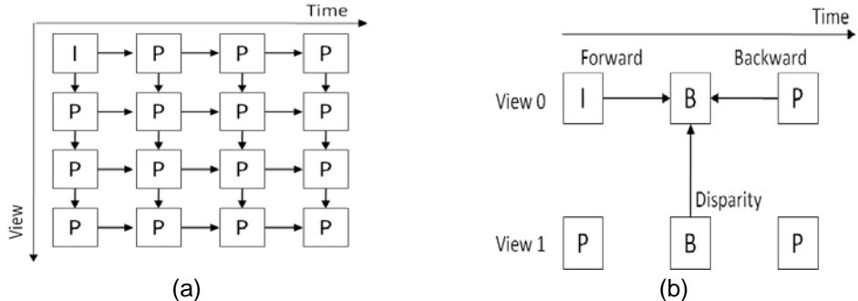
**Figure 3-16** a) Sequential view prediction structure using P-frames and b) prediction sources in HBP prediction architecture (Zhang et al., 2008; Chiang et al., 2011)
