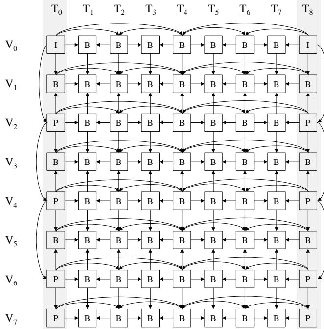
**Figure 2-6** Typical prediction architecture for multi-view video coding (Jeon et al., 2009)
