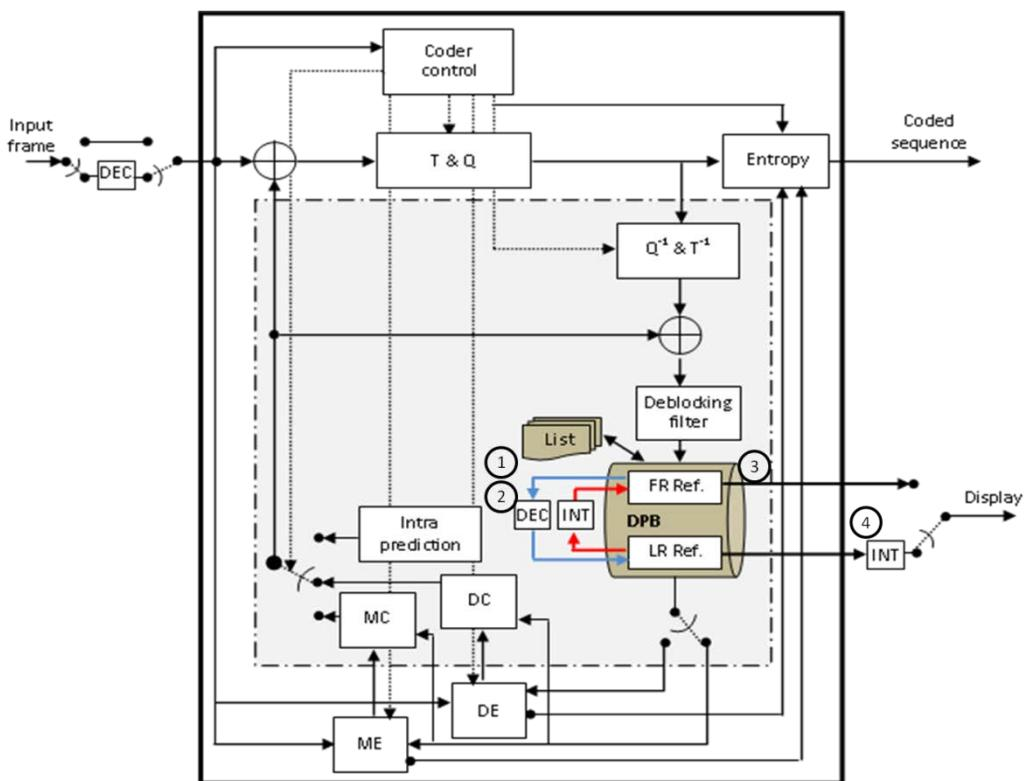
**Figure 5-1** Block diagram for the studies conducted in mixed spatial-resolution multi-view video coding
