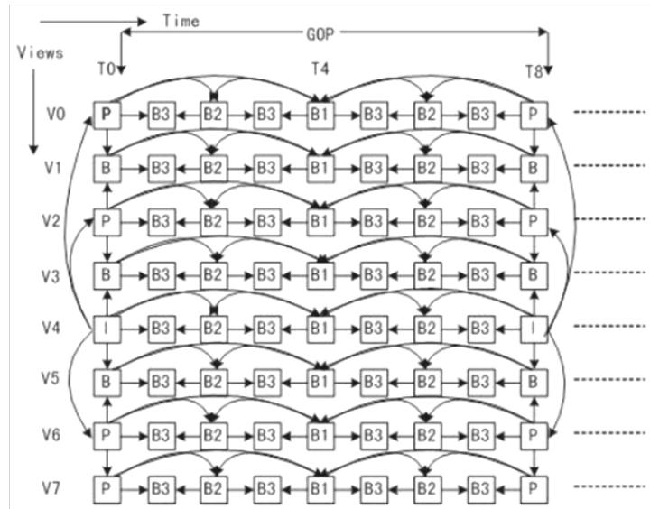
**Figure 3-6** HBP prediction architecture using middle view as base view (Lv, 2013)
