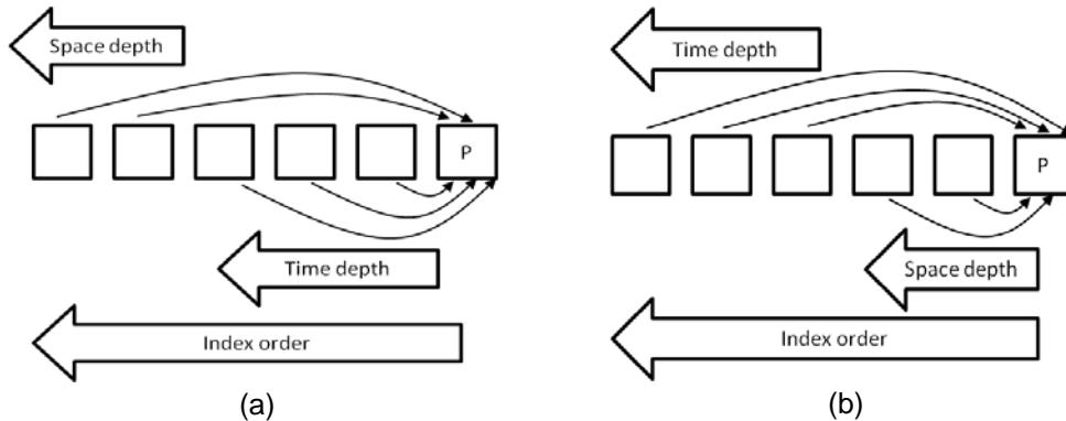
**Figure 3-15** Reference frame ordering used by *Sheikh Akbari et al.*, where a) temporal-first and b) spatial-first (Sheikh Akbari et al., 2007)
