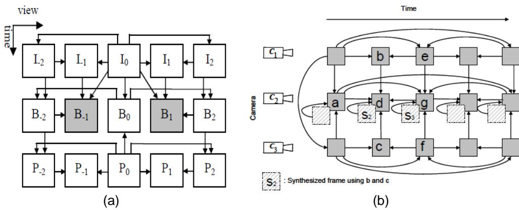
**Figure 3-8** Prediction architecture proposed by a) *An et al.* and b) *Pourazad et al.* (An et al., 2008; Pourazad et al., 2009a)
