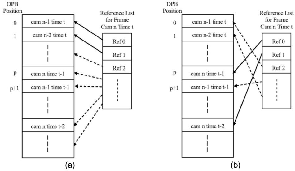
**Figure 3-14** Decoded picture buffer with reference frame ordering for a) opposite to coding order and b) temporal-first (Bilen et al., 2006)
