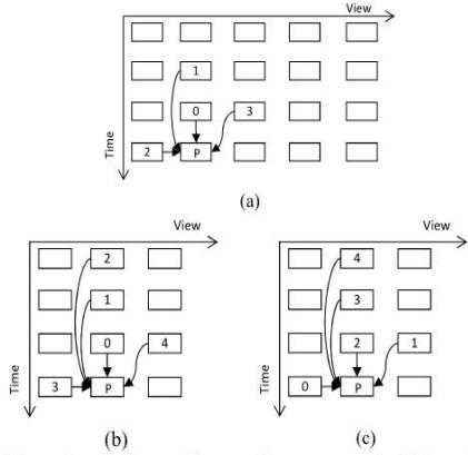
Figure 1-a Reference frame orders proposed by Bilen *et al.* (mode 3) [8], Figures 1-b and 1-c are modes 3 and mode 1 respectively that represent reference frame orders proposed by Sheikh Akbari *et al.* [10].
