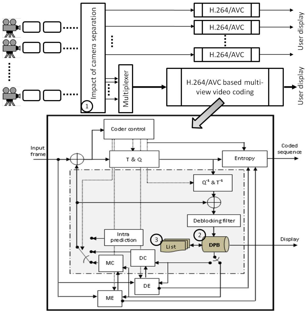
**Figure 4-1** Block diagram for the studies conducted in symmetric multi-view video coding
