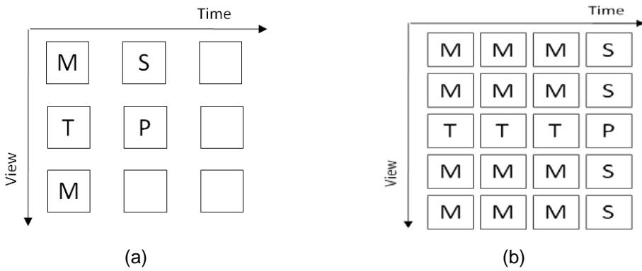
**Figure 3-4** Block matching analysis using a) Single temporal order and b) Higher temporal order (Merkle et al., 2006; Kaup & Fecker, 2006)
