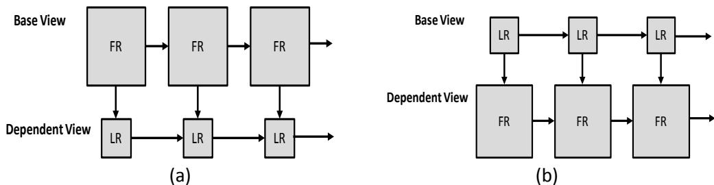
**Figure 5-5** Mixed spatial-resolution stereoscopic video codec with two different inter-view prediction directions, where base view is a) FR and b) LR
