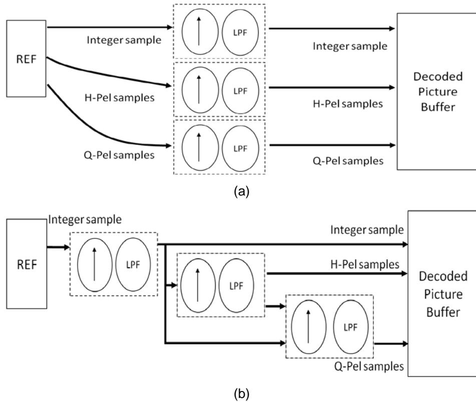
**Figure 5-16 (a-b)** Reference frame interpolation using conventional and high performance methods respectively
