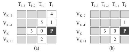
Figure 3. Proposed Reference frame architectures using: a) 6 reference frames and b) 4 reference frames.
