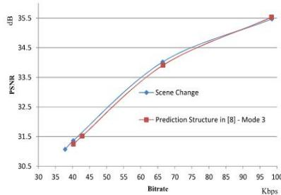
Figure 6. Coding performance for the proposed algorithm using the prediction structure proposed by Bilen *et al.* [8].
