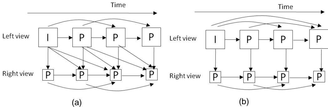
**Figure 3-20** Prediction architectures for stereoscopic video coding: a) mode 1 by *Bilen et al.* and b) 3D-DMB by *Fehn et al.* (Bilen et al., 2006; Fehn et al., 2007)
