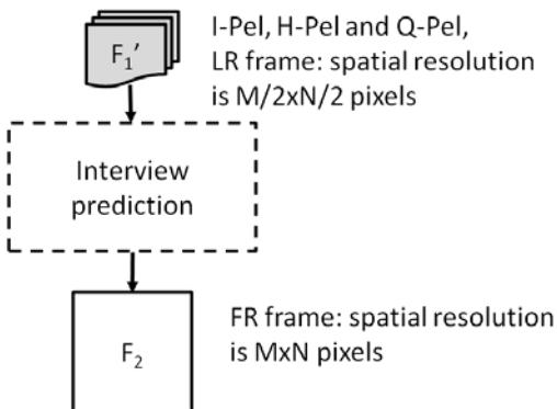
**Figure 5-15** Inter-view prediction using LR reference frame
