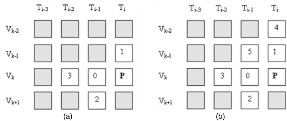
**Figure 4-18** The proposed prediction architectures using: a) 4 reference frames and b) 6 reference frames
