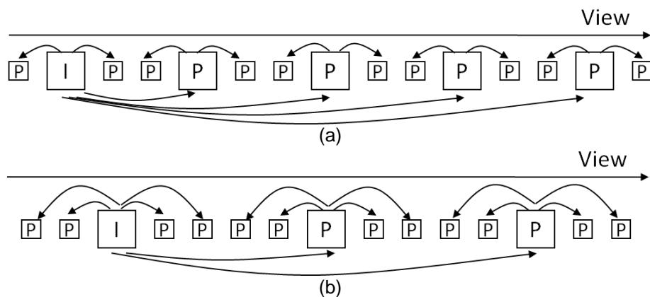
**Figure 3-24** Different configurations for inter-view prediction among anchor frames for GOV equal a) 3 and b) 5 (Ekmekcioglu et al., 2008a)
