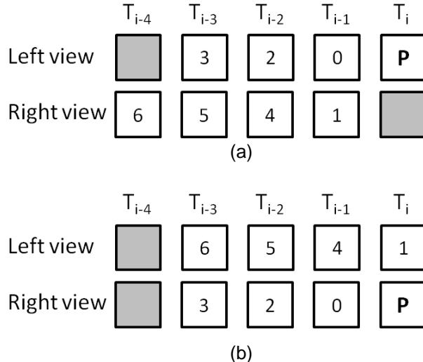
**Figure 4-13** Reference frame order (according to their block matching contribution among reference frames for coding frames a) left view and b) right view
