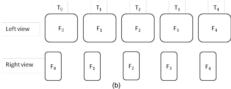
**Figure 3-25** Different down-sampling for right view a) vertical sampling and b) horizontal sampling (Yu et al., 2010)
