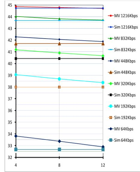
Fig. 4. Average PSNR<sub>Y</sub> for Simulcast and multi-view video codec at different bitrates and inter-camera angles.
