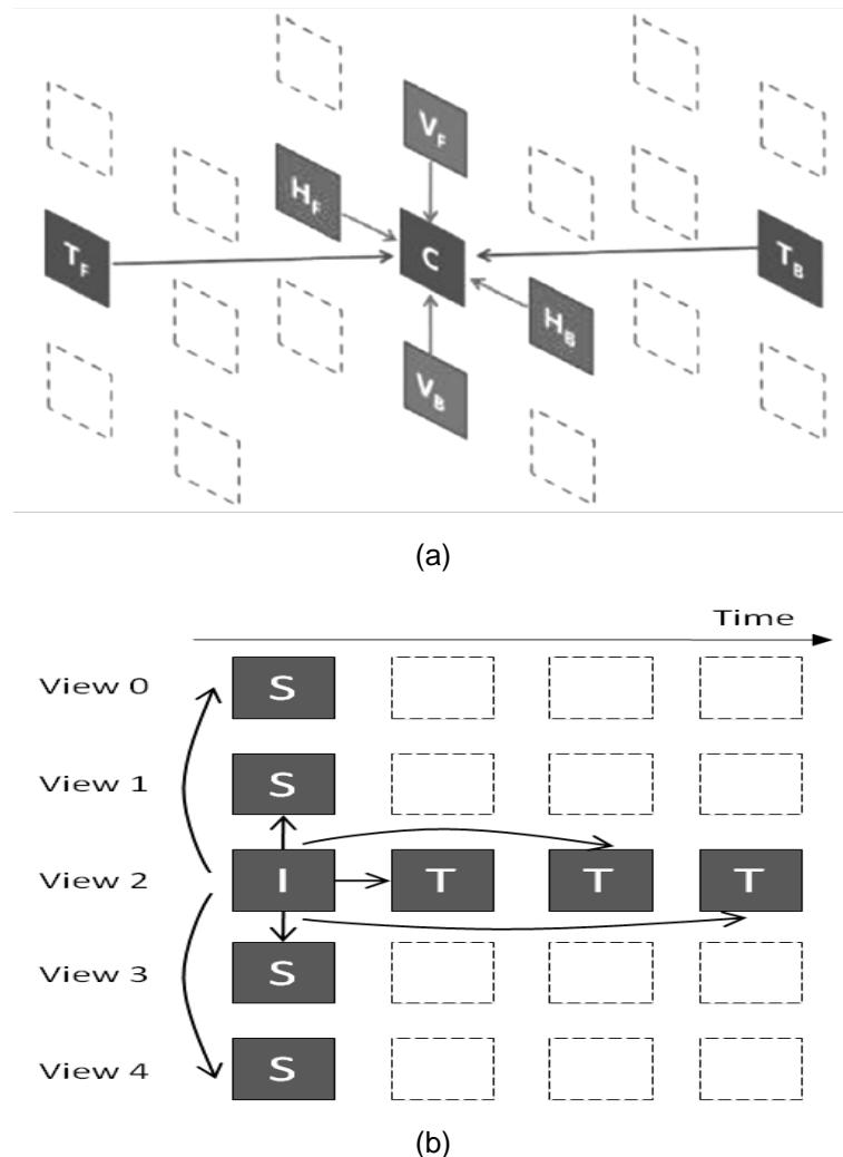
**Figure 3-3** Spatial-temporal correlation analysis using HBP a) 2-D camera array and b) 1-D camera array (Chung et al., 2008b; Zhang & Cai, 2011)
