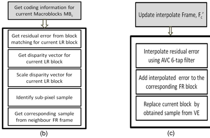
**Figure 5-40** Proposed visual enhancement algorithm: a) Main algorithm, b) Coding information utilisation and c) Frame update procedure
