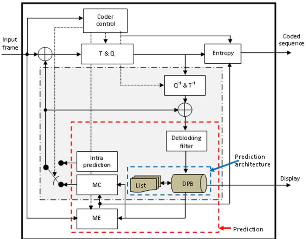
**Figure 2-1** H.264/AVC block diagram for monoscopic video coding (Schwarz et al., 2006; Richardson, 2010)
