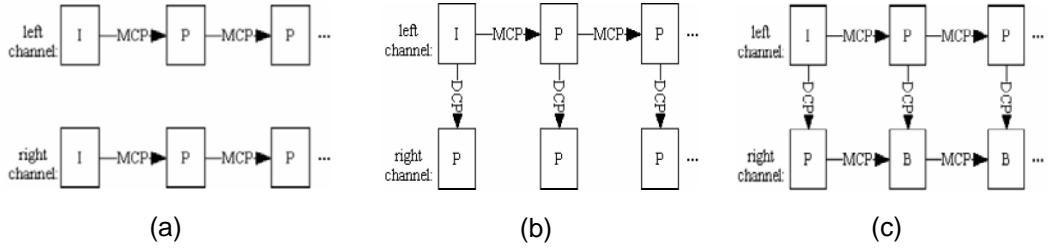
**Figure 3-10** Multiple schemes presented by *Li et al.*, where right frames use a) MCP, b) DCP and c) MCP and DCP (*Li et al.*, 2004)
