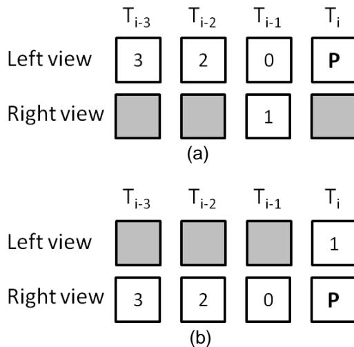
**Figure 4-14** Block diagram of the proposed prediction architecture for coding a) left view and b) right view
