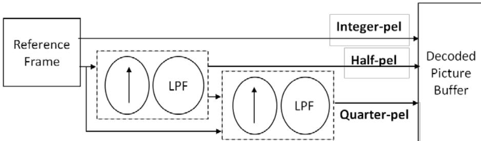
**Figure 2-4** Sub-pixel samples generation via H.264/AVC
