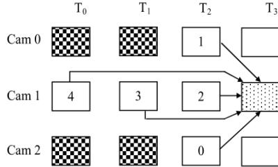
Fig. 3. Temporal and cross-view referencing for the proposed multi-view video codec.
