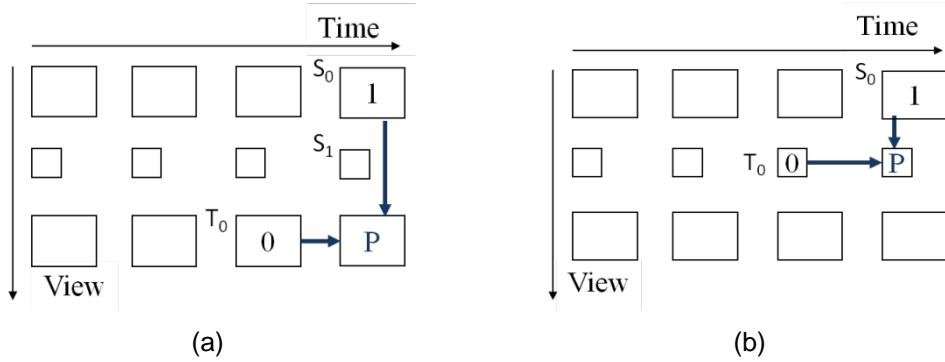
**Figure 5-21** Reference frame selection and reference frame ordering for a) full and b) low spatial-resolution frames
