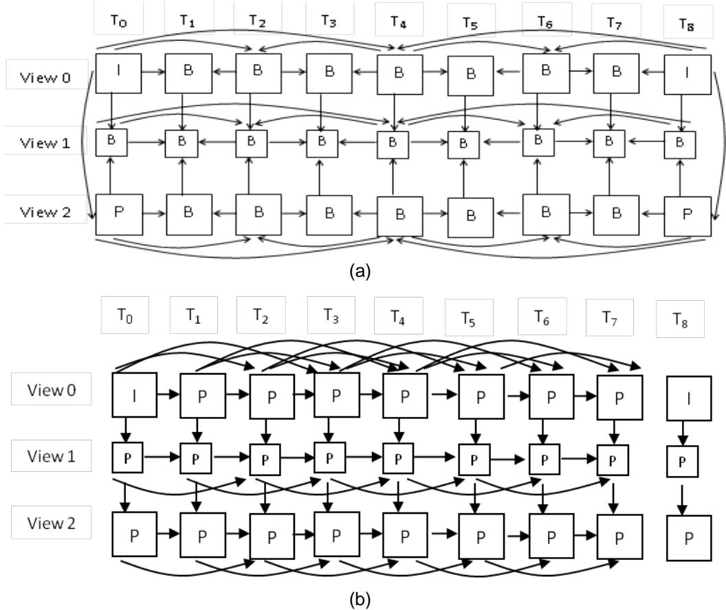
**Figure 5-28** Prediction architectures a) HBP and b) Extended prediction architecture based 3D-DMB (Chen et al., 2008a; Fehn et al., 2007)
