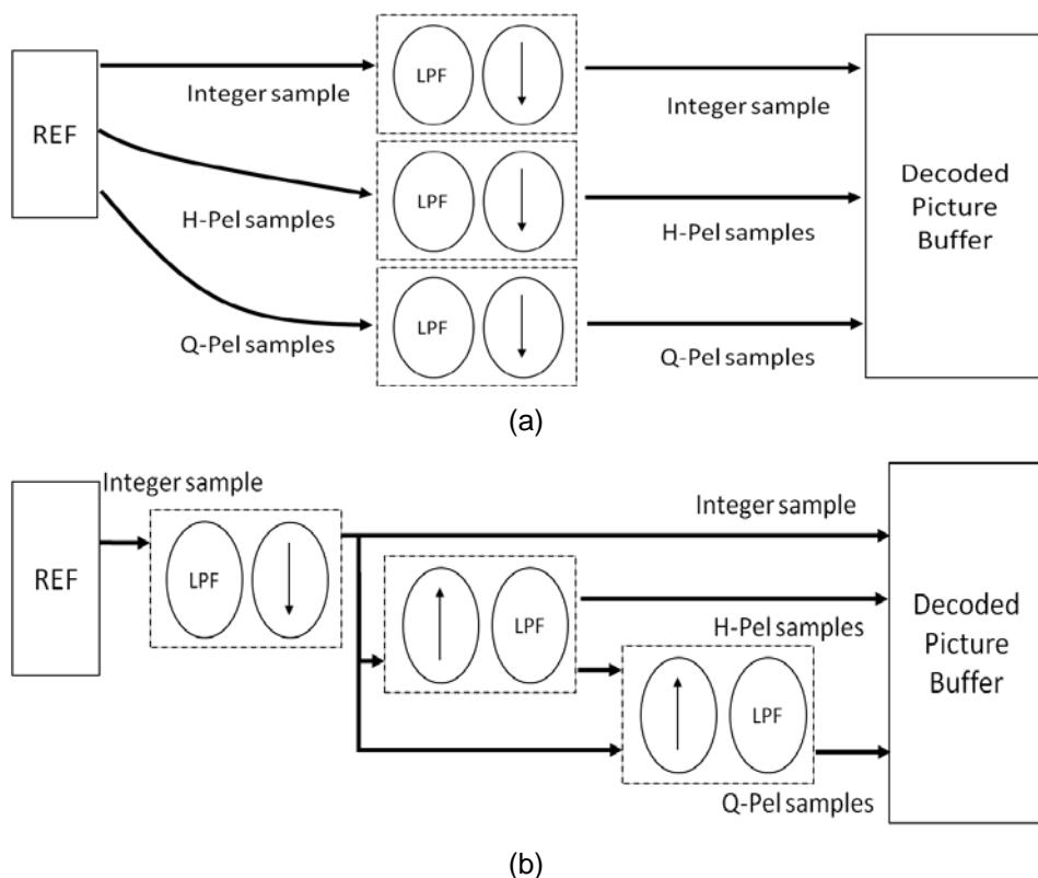
**Figure 5-11** Decimation methods a) conventional and b) high performance method
