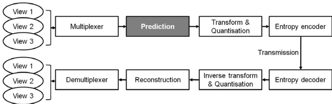
**Figure 1-2** General block diagram for H.264/AVC based multi-view video coding
