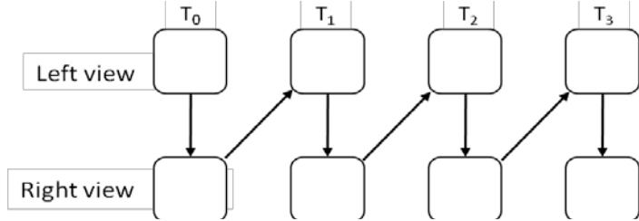
**Figure 4-10** Multiplexing frames generated from both cameras into single sequence
