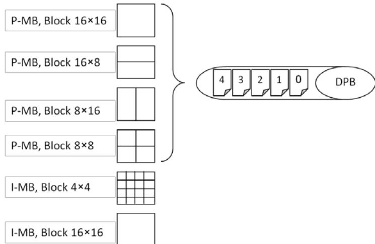
**Figure 2-5** Block matching process when number of reference frames is 5 (Yu-wen et al., 2006)
