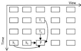
Figure 2 the prediction structure used in investigating reference frame order
