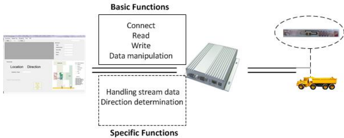
Figure 3- 7: Middleware Functions of RFID System
