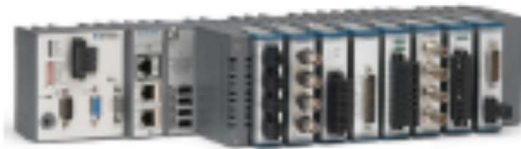
Figure 7.3: The cRIO-9024 real-time controller.
