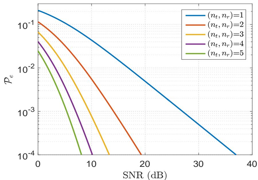
FIGURE 5.10: Probability of error for conventional transmission with one transmit-receive antennae pair and cooperative transmission for degree of diversity two, three, four and five.
