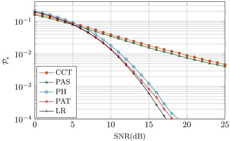
FIGURE 4.18: Performance comparison of the Proposed Adaptive Transmission (PAT), Proposed Antenna Selection (PAS) and Proposed Hybrid (PH) schemes with Lattice Reduction (LR) and Conventional Cooperative Transmission Schemes (CCT) for Minimum Mean Square Error (MMSE) detection with transmit and receive antennae are 8.
