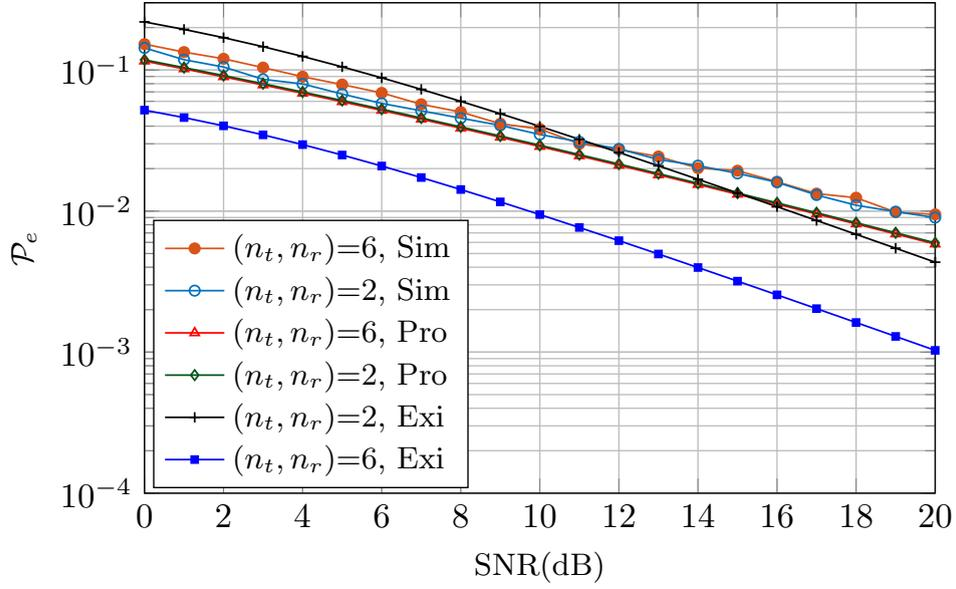
FIGURE 4.9: Error performance bound comparison of the Proposed (Pro) framework with Simulations (Sim) and Existing (Exi) frameworks for Minimum Mean Square Error (MMSE) detection, where transmit and receive antennae  $(n_t, n_r)$  are 2 and 6.
