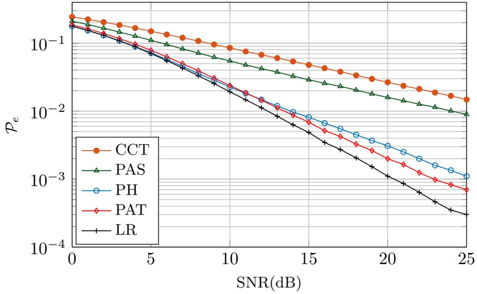
FIGURE 4.13: Performance comparison of the Proposed Adaptive Transmission (PAT), Proposed Antenna Selection (PAS) and Proposed Hybrid (PH) schemes with Lattice Reduction (LR) and Conventional Cooperative Transmission Schemes (CCT) for Zero Forcing (ZF) detection with transmit and receive antennae are 3.
