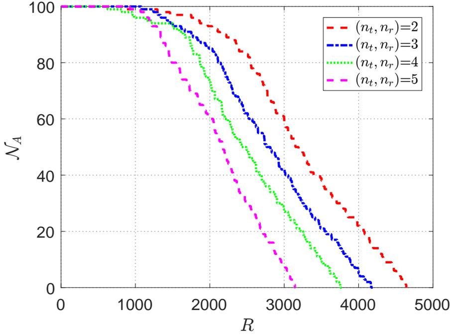
FIGURE 5.3: Performance analysis of the proposed scheme for cooperative communication realising virtual MIMO transmission and exploiting diversity for number of alive nodes  $\mathcal{N}_A$  and rounds  $R$ .
