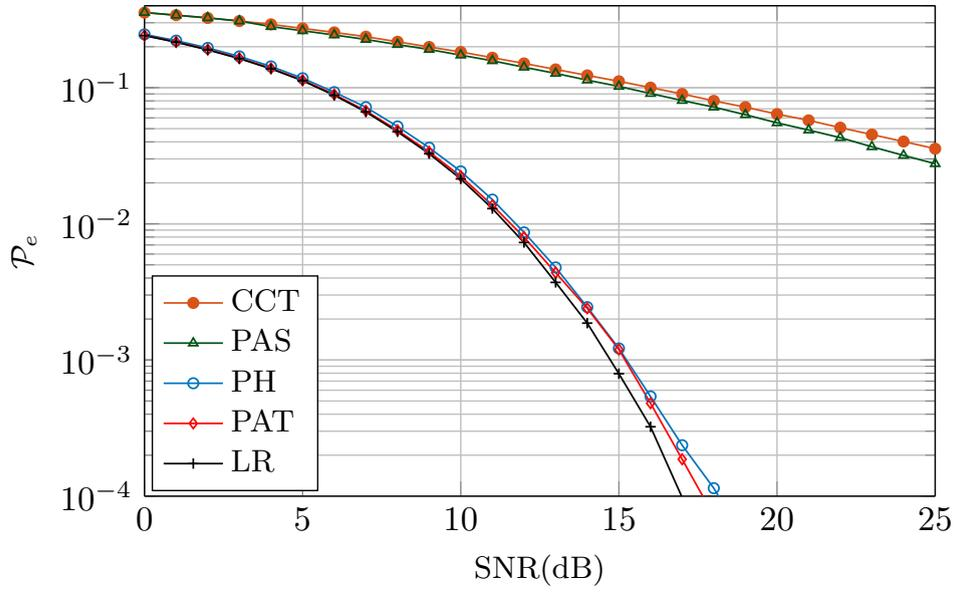
FIGURE 4.19: Performance comparison of the Proposed Adaptive Transmission (PAT), Proposed Antenna Selection (PAS) and Proposed Hybrid (PH) schemes with Lattice Reduction (LR) and Conventional Cooperative Transmission Schemes (CCT) for Zero Forcing (ZF) detection with transmit and receive antennae are 10.
