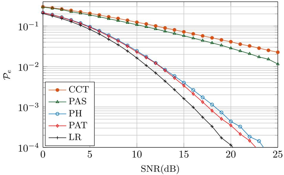
FIGURE 4.15: Performance comparison of the Proposed Adaptive Transmission (PAT), Proposed Antenna Selection (PAS) and Proposed Hybrid (PH) schemes with Lattice Reduction (LR) and Conventional Cooperative Transmission Schemes (CCT) for Zero Forcing (ZF) detection with transmit and receive antennae are 5.
