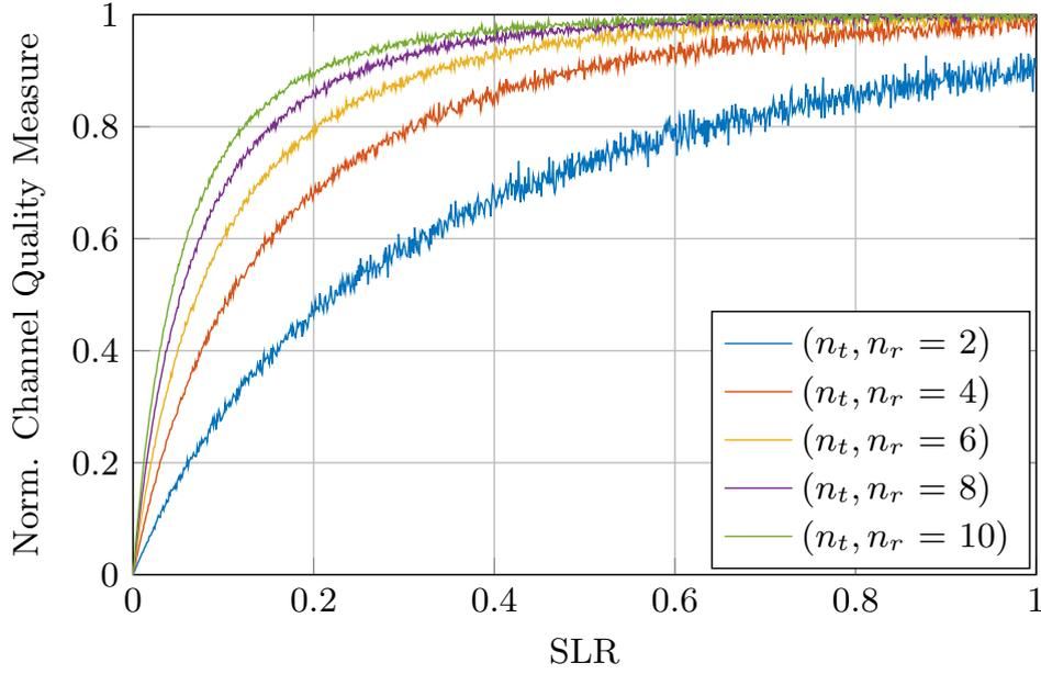
FIGURE 4.5: Normalised channel quality measure for  $(n_t, n_r) = 2, 4, 6, 8$  and  $10$ .
