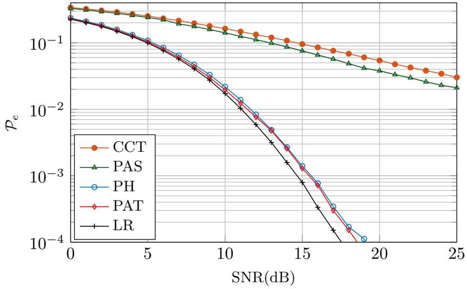
FIGURE 4.17: Performance comparison of the Proposed Adaptive Transmission (PAT), Proposed Antenna Selection (PAS) and Proposed Hybrid (PH) schemes with Lattice Reduction (LR) and Conventional Cooperative Transmission Schemes (CCT) for Zero Forcing (ZF) detection with transmit and receive antennae are 8.
