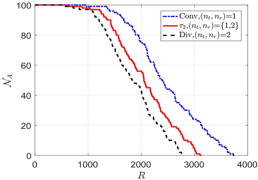
FIGURE 5.14: Performance comparison of the proposed universal framework channel quality index (CQI) based adaptation  $(n_t, n_r) = \{1,2\}$ , conventional cooperative transmission  $(n_t, n_r) = 1$  and virtual MIMO diversity for  $(n_t, n_r) = 2$  for number of alive nodes  $\mathcal{N}_A$  and rounds  $R$ .
