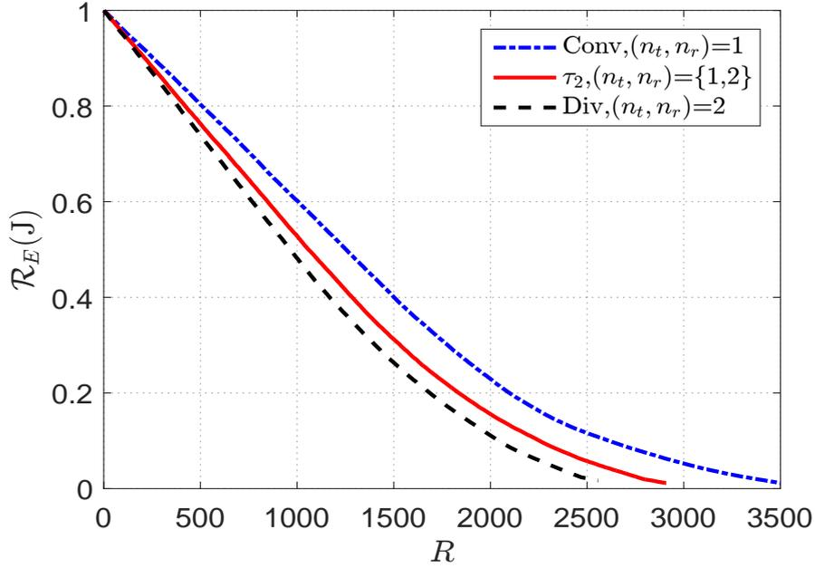
FIGURE 5.15: Performance comparison of the proposed universal framework channel quality index (CQI) based adaptation  $(n_t, n_r) = \{1,2\}$ , conventional cooperative transmission  $(n_t, n_r) = 1$  and virtual MIMO diversity for  $(n_t, n_r) = 2$  for average residual energy  $\mathcal{R}_E$  and rounds  $R$ .
