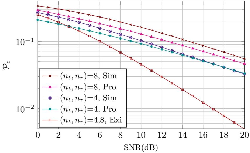
FIGURE 4.8: Error performance bound comparison of the Proposed (Pro) framework with Simulations (Sim) and Existing (Exi) frameworks for Zero Forcing (ZF) detection, where transmit and receive antennae  $(n_t, n_r)$  are 4 and 8.
