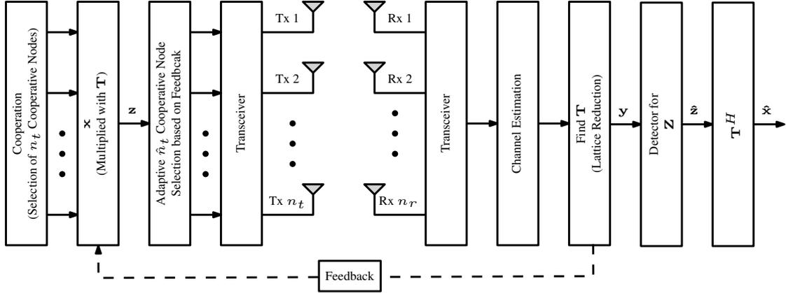
FIGURE 4.3: Block diagram summarising the methodological steps of the MIMO system with lattice reduction aided data detection.
