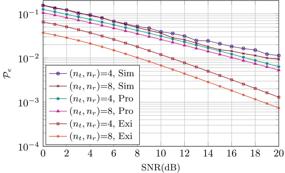
FIGURE 4.10: Error performance bound comparison of the Proposed (Pro) framework with Simulations (Sim) and Existing (Exi) frameworks for Minimum Mean Square Error (MMSE) detection, where transmit and receive antennae  $(n_t, n_r)$  are 4 and 8.
