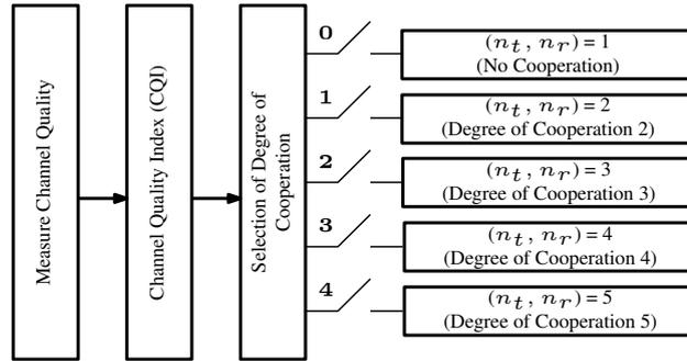
FIGURE 5.2: Block Diagram for Channel Quality Index.
