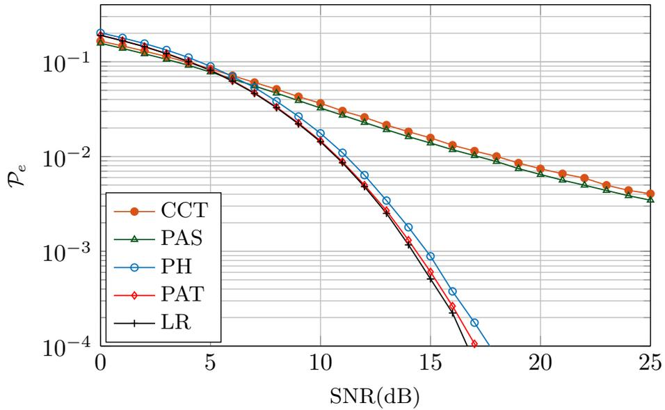
FIGURE 4.20: Performance comparison of the Proposed Adaptive Transmission (PAT), Proposed Antenna Selection (PAS) and Proposed Hybrid (PH) schemes with Lattice Reduction (LR) and Conventional Cooperative Transmission Schemes (CCT) for Minimum Mean Square Error (MMSE) detection with transmit and receive antennae are 10.
