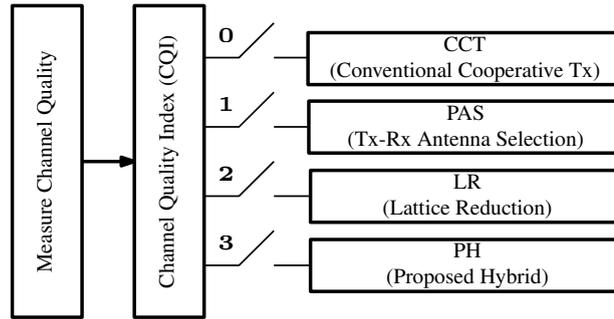
FIGURE 4.4: Block diagram for the channel quality index.
