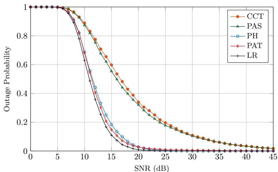
FIGURE 4.27: Outage Probability comparison of the Proposed Adaptive Transmission (PAT), Proposed Antenna Selection (PAS), Proposed Hybrid (PH) schemes with Lattice Reduction (LR) and Conventional Cooperative Transmission (CCT) schemes, where transmit and receive antennae are five.
