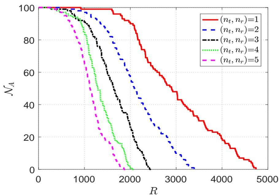
FIGURE 5.6: Performance analysis of the proposed scheme for event-driven applications for the number of alive nodes  $\mathcal{N}_A$  and rounds  $R$ .
