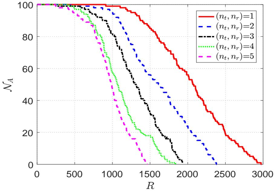
FIGURE 5.4: Performance analysis of the proposed scheme for time-driven applications for the number of alive nodes  $\mathcal{N}_A$  and rounds  $R$ .
