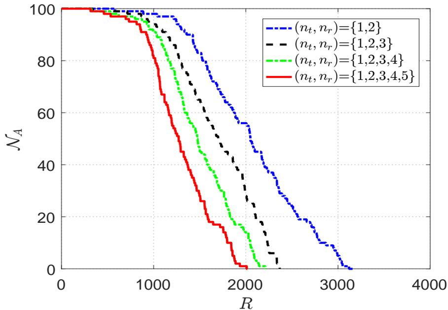
FIGURE 5.12: Performance analysis of the proposed universal framework with channel quality index (CQI) based adaptation for number of alive nodes  $\mathcal{N}_A$  and rounds  $R$ .
