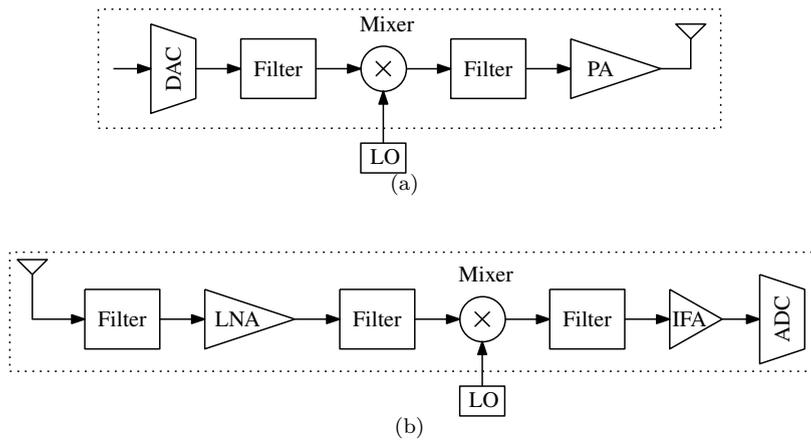
FIGURE 3.4: (a) Transmitter circuit blocks, (b) Receiver circuit blocks.
