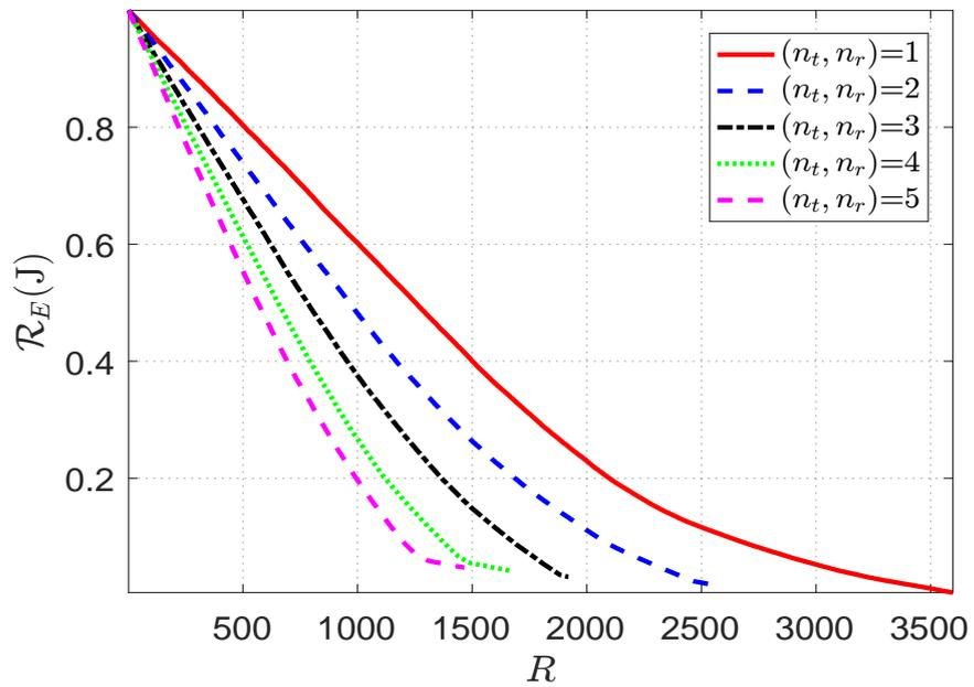
FIGURE 5.9: Performance analysis of the proposed scheme for hybrid applications for the average residual energy  $\mathcal{R}_E$  and rounds  $R$ .
