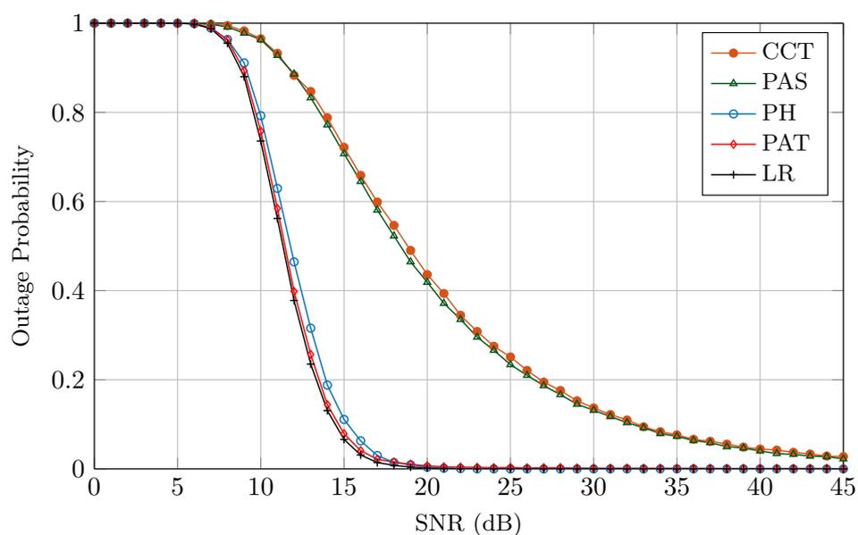
FIGURE 4.28: Outage Probability comparison of the Proposed Adaptive Transmission (PAT), Proposed Antenna Selection (PAS), Proposed Hybrid (PH) schemes with Lattice Reduction (LR) and Conventional Cooperative Transmission (CCT) schemes, where transmit and receive antennae are eight.
