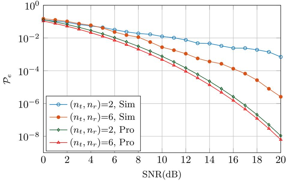
FIGURE 4.11: Error performance bound comparison of the Proposed (Pro) framework with Simulations (Sim) and Existing (Exi) frameworks for Maximum Likelihood (ML) detection, where transmit and receive antennae  $(n_t, n_r)$  are 2 and 6.
