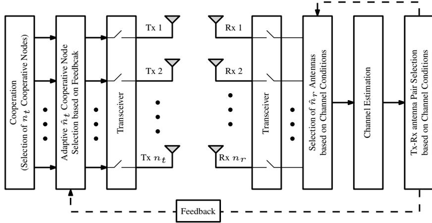
FIGURE 4.2: Block diagram of the proposed Tx-Rx antennae selection for cooperative communication within WSNs.
