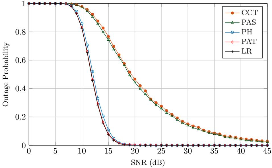
FIGURE 4.29: Outage Probability comparison of the Proposed Adaptive Transmission (PAT), Proposed Antenna Selection (PAS), Proposed Hybrid (PH) schemes with Lattice Reduction (LR) and Conventional Cooperative Transmission (CCT) schemes, where transmit and receive antennae are ten.
