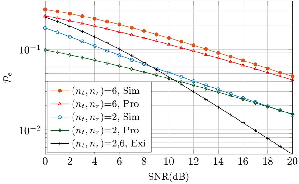
FIGURE 4.7: Error performance bound comparison of the Proposed (Pro) framework with Simulations (Sim) and Existing (Exi) frameworks for Zero Forcing (ZF) detection, where transmit and receive antennae  $(n_t, n_r)$  are 2 and 6.
