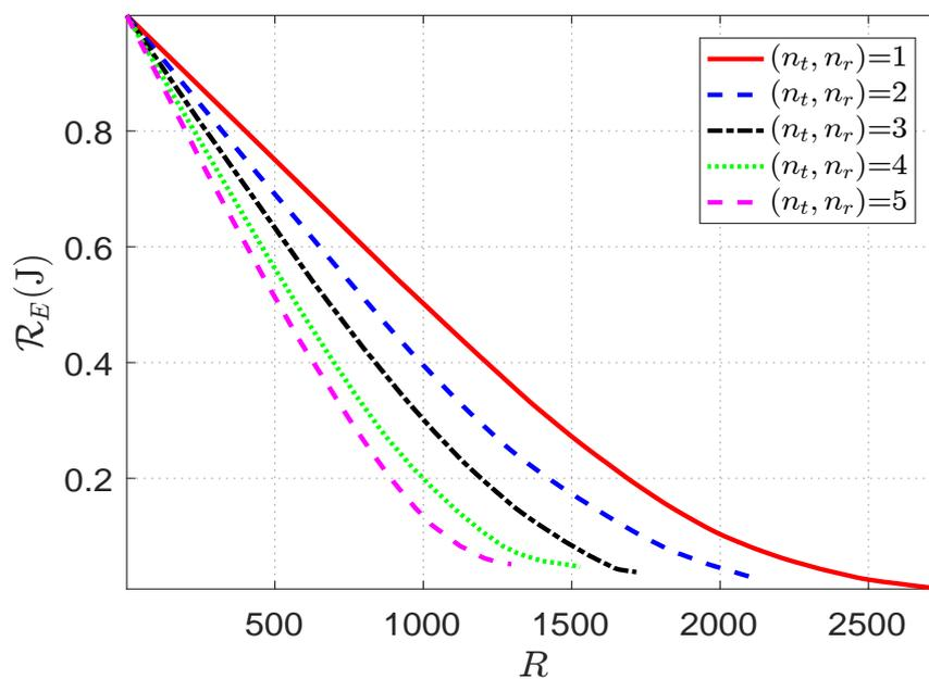
FIGURE 5.5: Performance analysis of the proposed scheme for time-driven applications for the average residual energy  $\mathcal{R}_E$  and rounds  $R$ .
