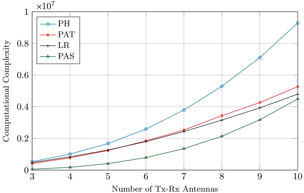
FIGURE 4.25: Computational complexity comparison of the Proposed Adaptive Transmission (PAT), Proposed Antennae Selection (PAS), Proposed Hybrid (PH) schemes with Lattice Reduction (LR) where the network size is 1500.
