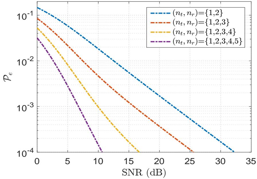
FIGURE 5.11: Probability of error for cooperative transmission with channel quality index (CQI) based adaptation for degree of diversity two, three, four and five.
