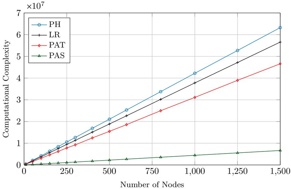
FIGURE 4.21: Computational complexity comparison of the Proposed Adaptive Transmission (PAT), Proposed Antenna Selection (PAS), Proposed Hybrid (PH) schemes with Lattice Reduction (LR) where transmit and receive antennae are three.
