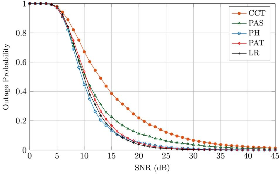
FIGURE 4.26: Outage Probability comparison of the Proposed Adaptive Transmission (PAT), Proposed Antenna Selection (PAS), Proposed Hybrid (PH) schemes with Lattice Reduction (LR) and Conventional Cooperative Transmission (CCT) schemes, where transmit and receive antennae are three.
