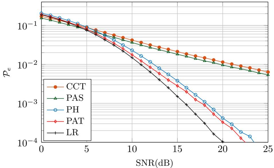
FIGURE 4.16: Performance comparison of the Proposed Adaptive Transmission (PAT), Proposed Antenna Selection (PAS) and Proposed Hybrid (PH) schemes with Lattice Reduction (LR) and Conventional Cooperative Transmission Schemes (CCT) for Minimum Mean Square Error (MMSE) detection with transmit and receive antennae are 5.
