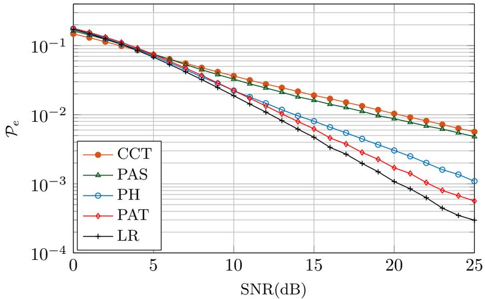
FIGURE 4.14: Performance comparison of the Proposed Adaptive Transmission (PAT), Proposed Antenna Selection (PAS) and Proposed Hybrid (PH) schemes with Lattice Reduction (LR) and Conventional Cooperative Transmission Schemes (CCT) for Minimum Mean Square Error (MMSE) detection with transmit and receive antennae are 3.
