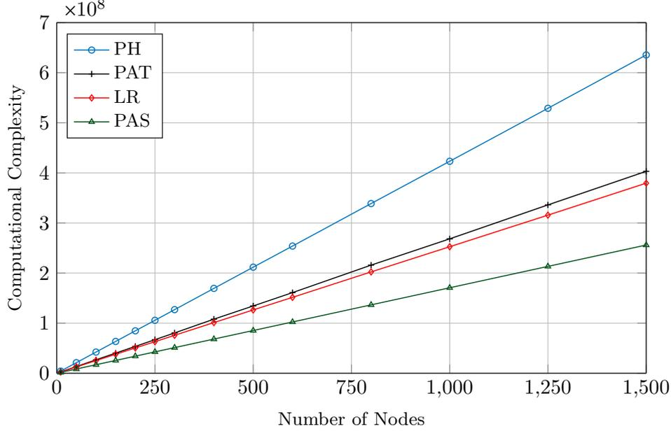
FIGURE 4.23: Computational complexity comparison of the Proposed Adaptive Transmission (PAT), Proposed Antenna Selection (PAS), Proposed Hybrid (PH) schemes with Lattice Reduction (LR) where transmit and receive antennae are eight.
