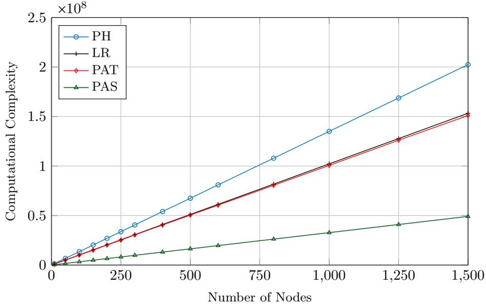
FIGURE 4.22: Computational complexity comparison of the Proposed Adaptive Transmission (PAT), Proposed Antenna Selection (PAS), Proposed Hybrid (PH) schemes with Lattice Reduction (LR) where transmit and receive antennae are five.
