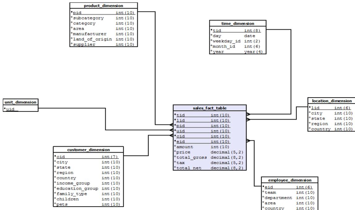
Figure 7-3: DM Star Schema based on MLED\_BI approach
