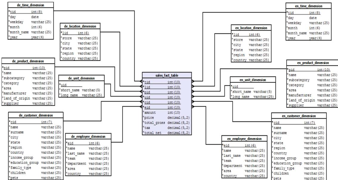
Figure 7-6: DM Star Schema based on ATS approach
