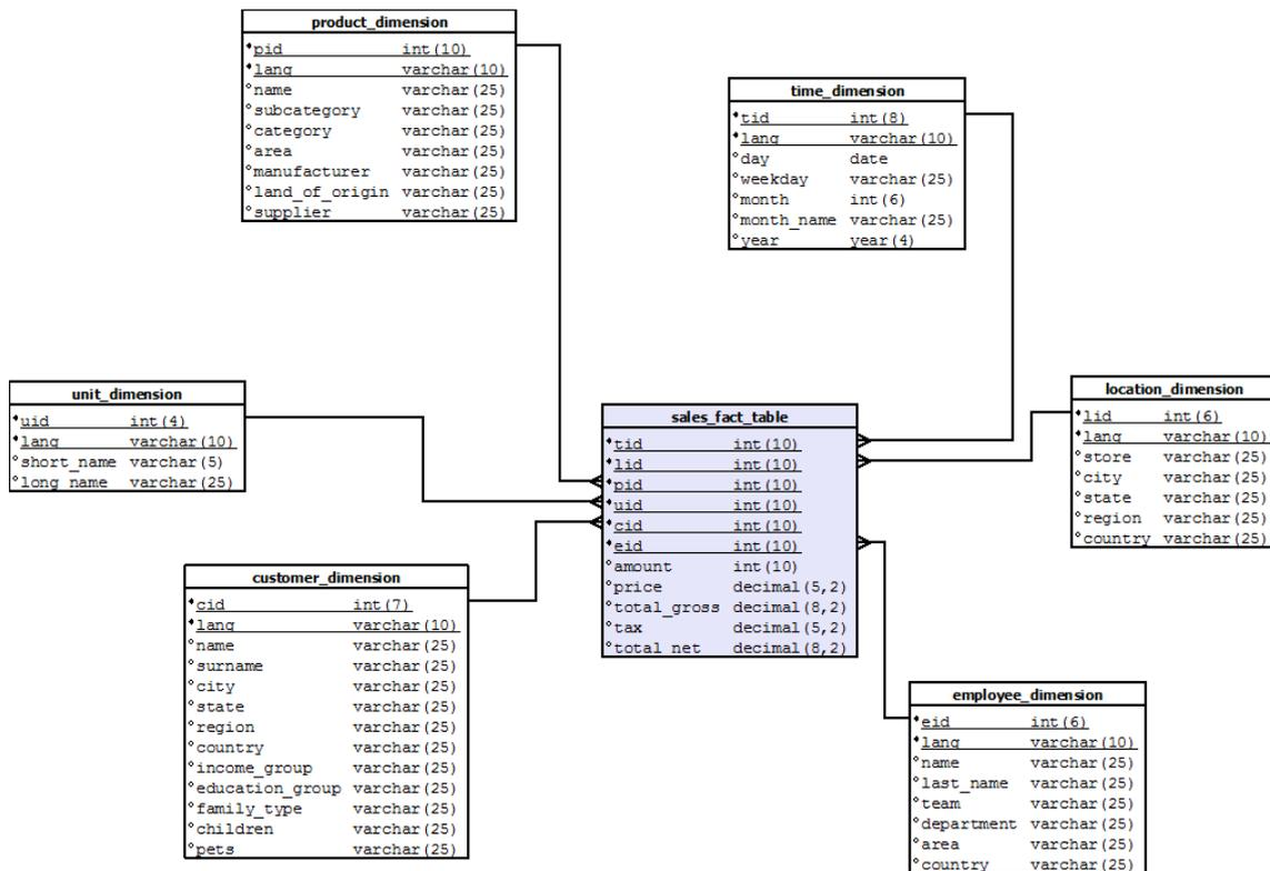
Figure 7-5: DM Star Schema based on the LIF approach
