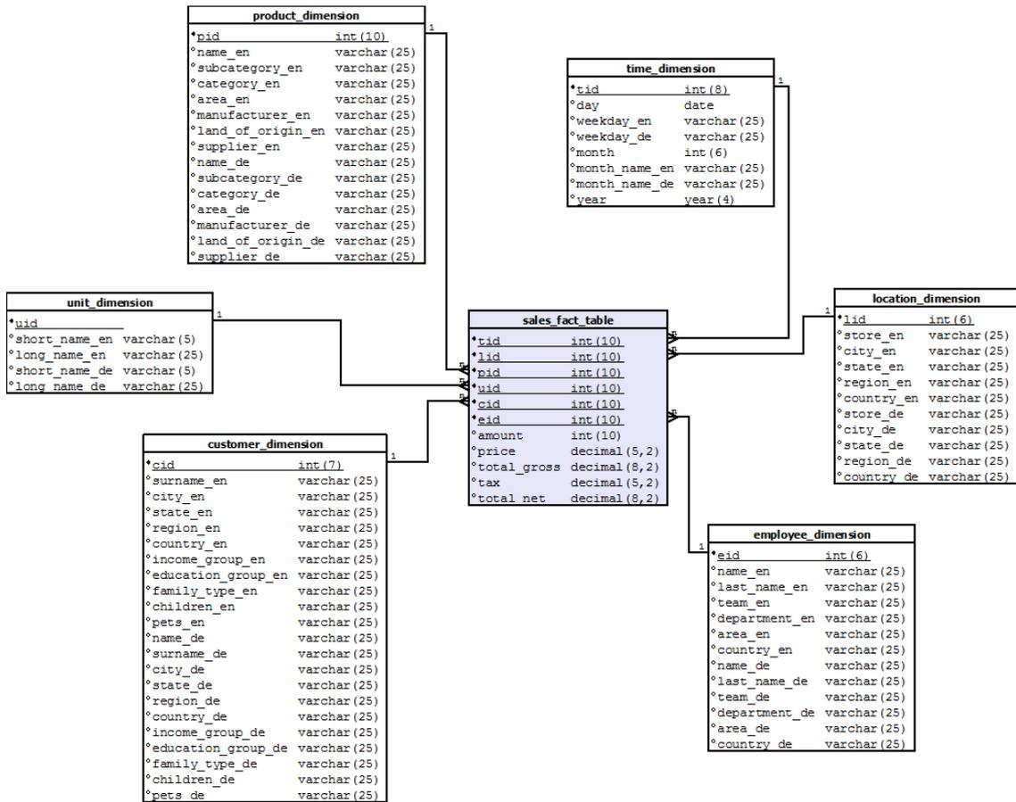
Figure 7-4: DM star schema based on the AA approach
