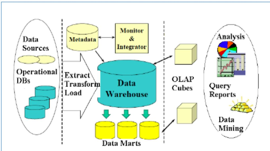
Figure A-9: Conventional BI Infrastructure according to Chu (2013, p. 114)
