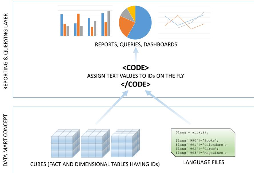
Figure 4-6: The process of assigning descriptions of attributes and hierarchies on the fly
