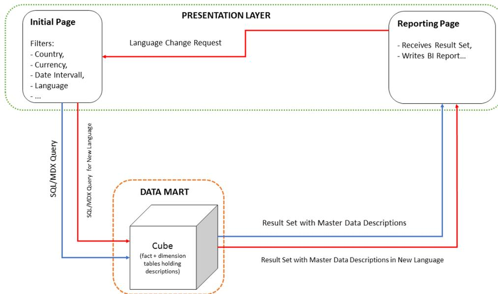
Figure 5-9: Architecture diagram showing the LIF PoC
