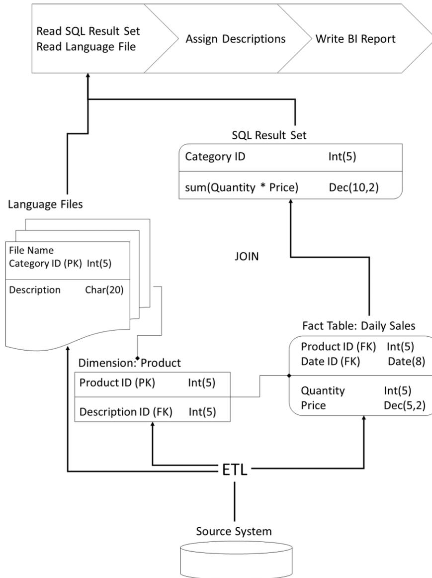
Figure 5-5: High-level overview of the physical design of the PoC artefact
