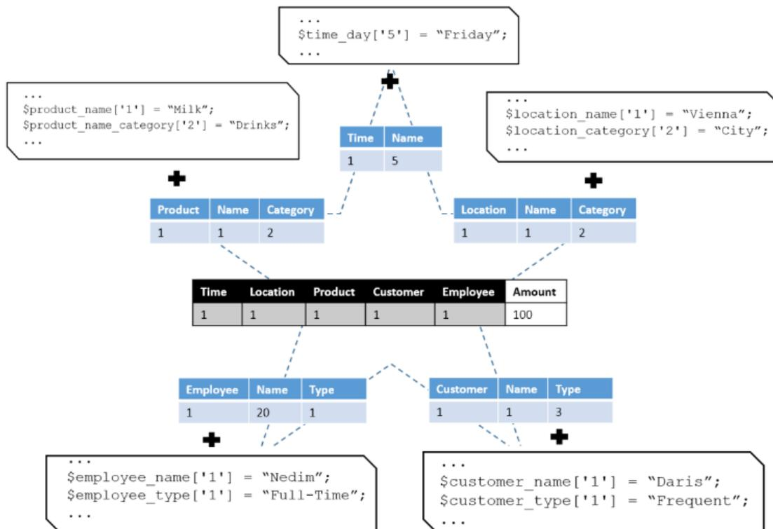
Figure 4-3: Data mart design based on MLED\_BI approach
