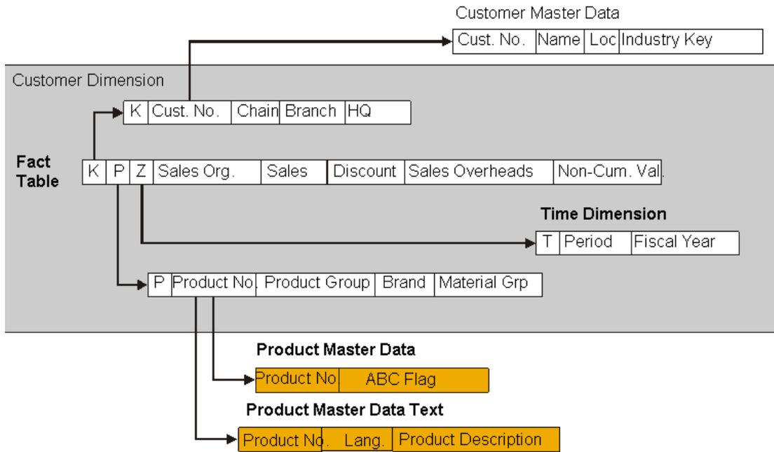
Figure 2-8: SAP BW extended star schema (Source: SAP, 2015)
