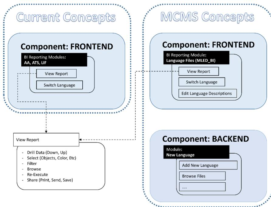
Figure 4-7: Comparison of conventional reporting layer functionality and functionality provided by a MCMS supported by MLED\_BI
