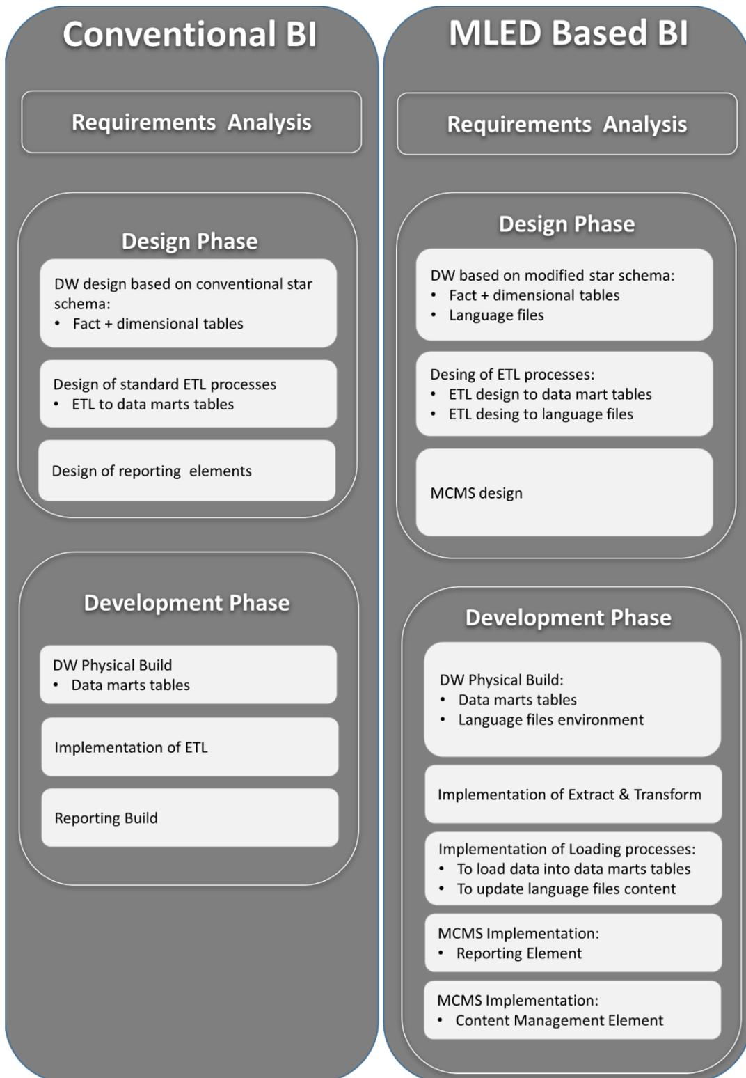
Figure 4-12: Differences in development phases between established BI design approaches and MLED\_BI
