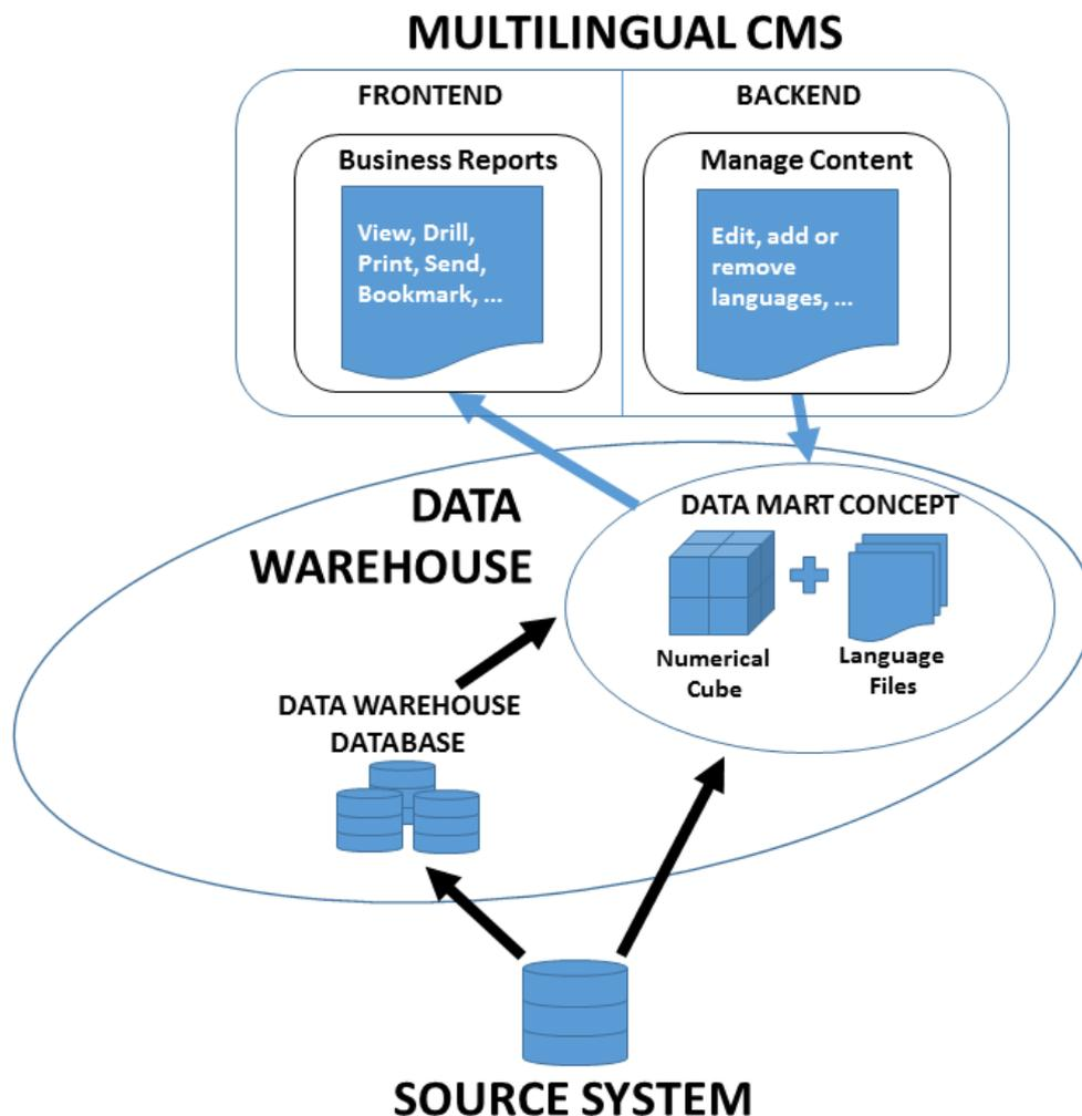
Figure 4-9: BI environment based on the MLED\_BI BI design approach
