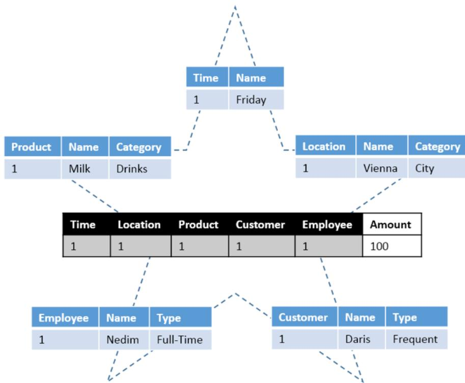
Figure 4-2: Data mart design based on the established Star schema approach
