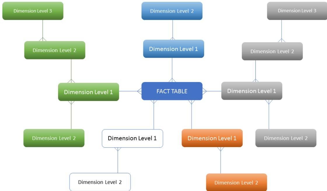
Figure 2-6: Representation of a Snowflake Schema
