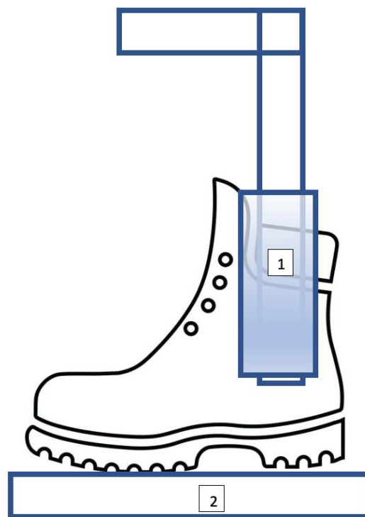
Figure 6-20 Positioning of ankle shank rotating frame in test footwear, (1) Shank ankle representative model, 2 Torque measurement footwear support platform
