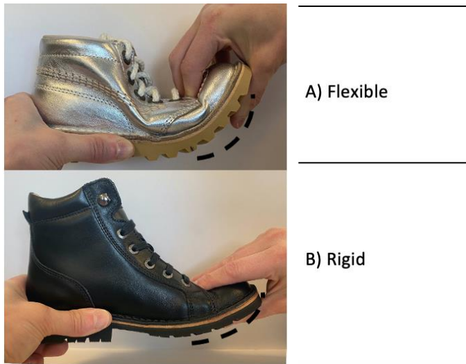
Figure 6 How to describe outsole flexibility in the toe spring and forefoot (A) Flexible (B) Rigid
