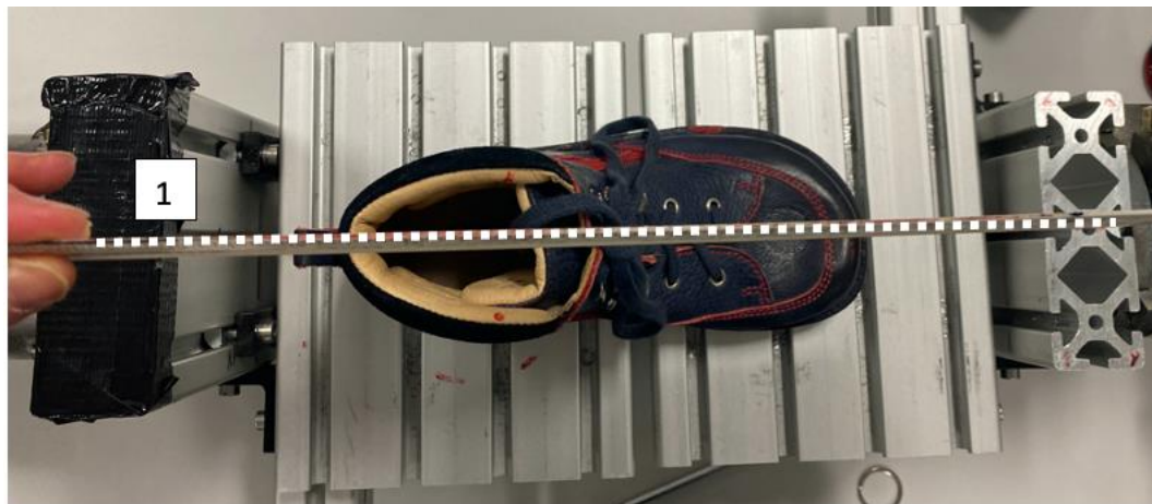
Figure 6-14 Alignment of the long axis of the footwear along the axis of the rotating system 1 Axis of the rotating system
