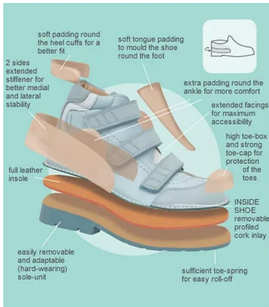
Figure 1-1 Standard construction of Off-the-Shelf stability clinical footwear Intervention (Source www.piedro-therapy.com/children ).
