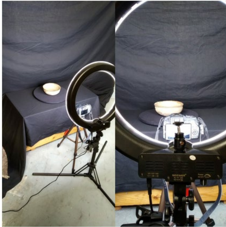
Fig. 37. Photogrammetry setup at the location for the Thornhill Collection, featuring the Green Glazed Bowl from the collection.
