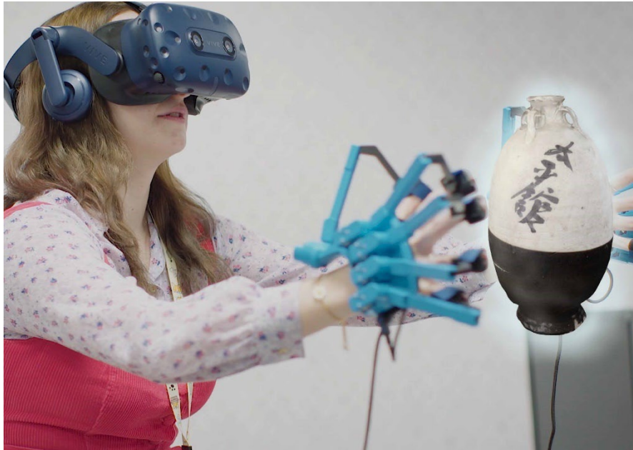
Fig. 30. Set up of the SenseGlove haptic gloves with the HTC Vive headset.
