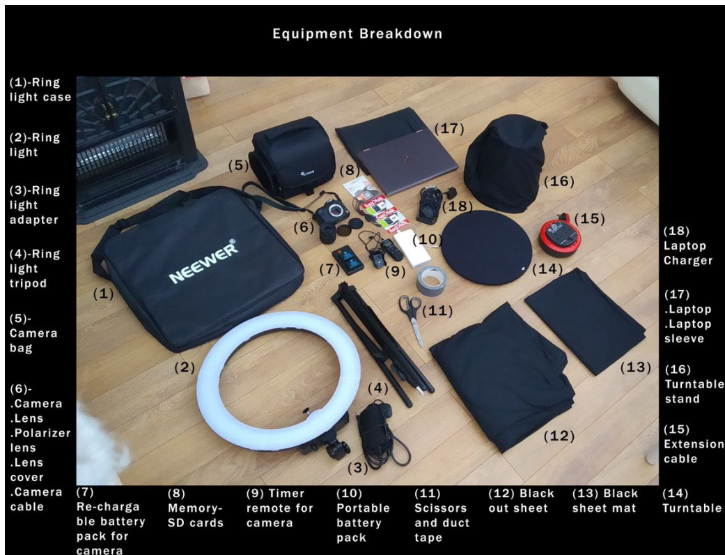
Fig. 38. Breakdown of Photogrammetry equipment.
