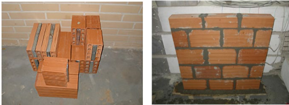
Fig. 2.12 Macro-encapsulated material within the red bricks (Rathore et al., 2019).
