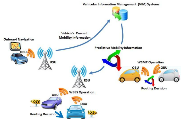
Figure 1. Proposed network architecture of the predictive routing for vehicular communication
