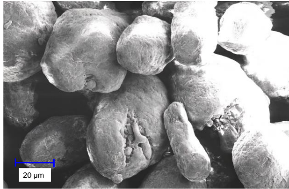
Fig. 12. Scanning electron microscope (SEM) image of SLS Aged PA12 showing details of the particles on the surface, as well as their different sizes and shapes.
