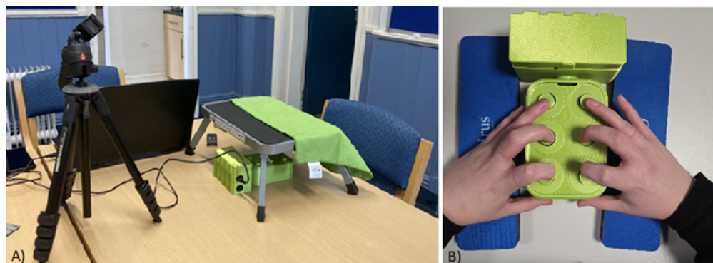
Figure 2. Experimental setting (A). The multisensory device was placed underneath a small table. Children were asked to place their fingers on the buttons (B), to be able to feel the haptic vibrations. Thumbs were placed on the start and cancel button.
