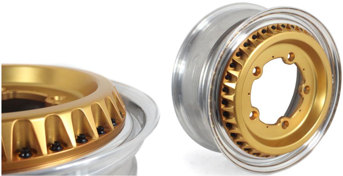
Figure 1. Three-piece aluminium wheel example (picture used with Company A permission).
