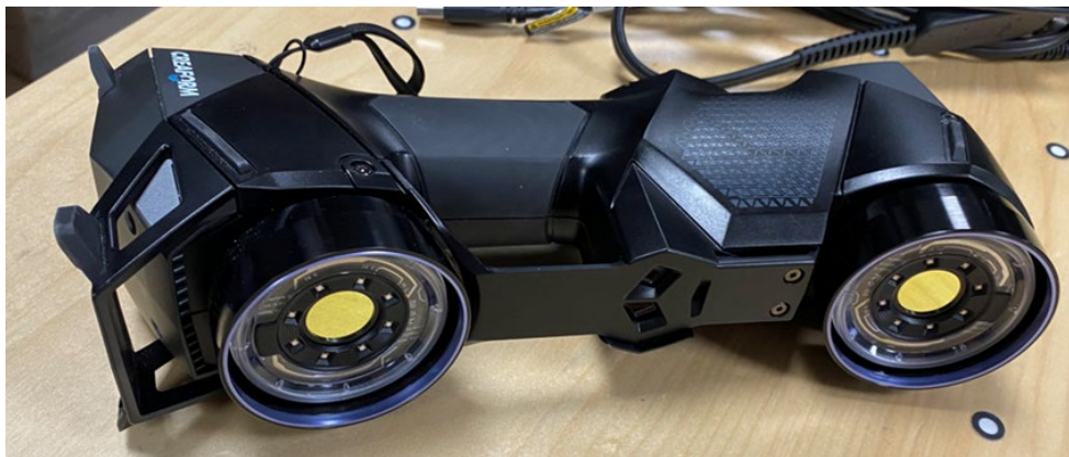
Figure 3.13 - HandyScan laser scanner. (Copyright: Alex Haycock)
