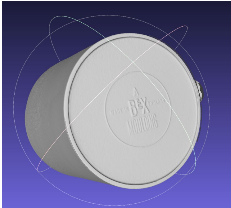
Figure 4.7: 3D laser scan of a pink plastic Passover cup demonstrating the detections of key details present on the object. (Copyright: Alex Haycock)
