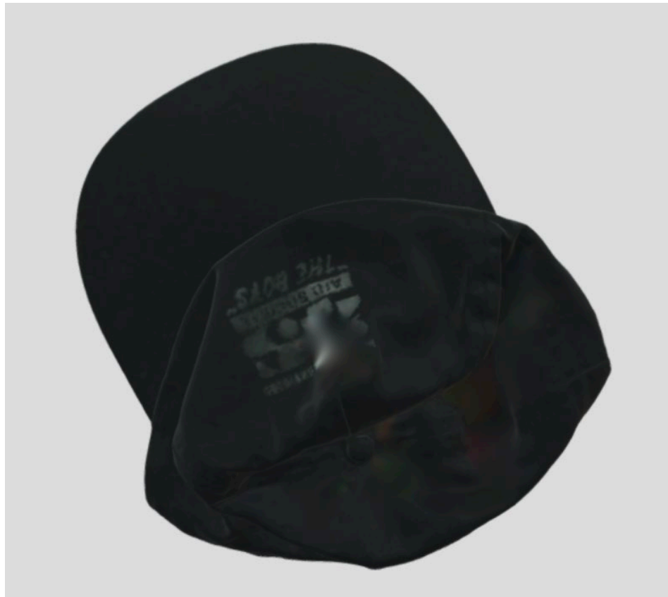
Figure 4.5: Structured light scan of a 45 Aid society cap. Due to the object being a dark material, some detail from the object is lost or hard to see. (Copyright: Alex Haycock)
