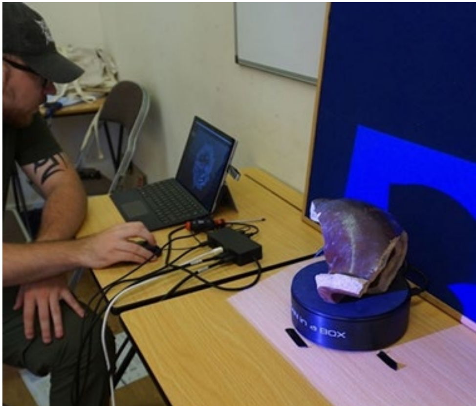
Figure 3.10 - Scan in a box FX Structured light scan in progress on an excavated object from the LDHP excavations. (Copyright: Alex Haycock)
