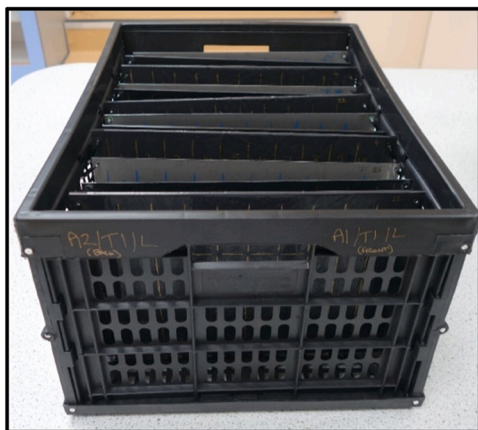
Fig. 2. Samples secured into a crate before submersion into the lake.
