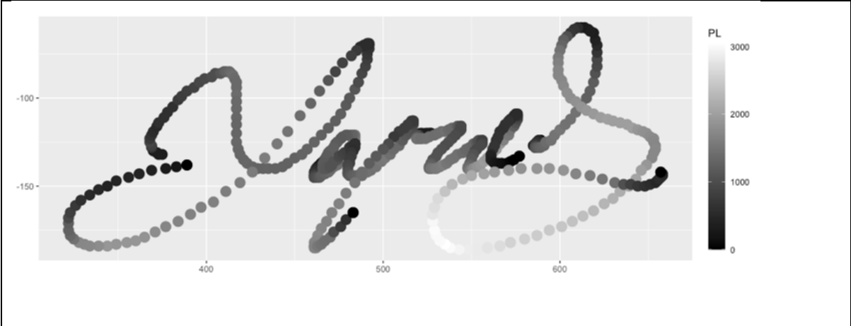
Figure 5.4 a. The reference DCS, captured with the target solution. pressure levels are represented as shades of grey, with black for 0 and white for the maximum pressure level value.
