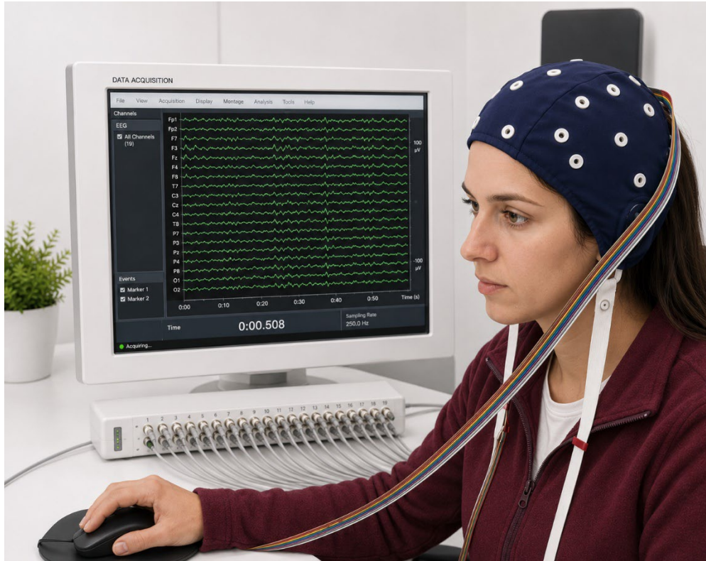
Figure 2.3: Illustration of an EEG system setup showing a participant wearing an electrode cap connected to a data acquisition unit displaying multi-channel EEG signals.
