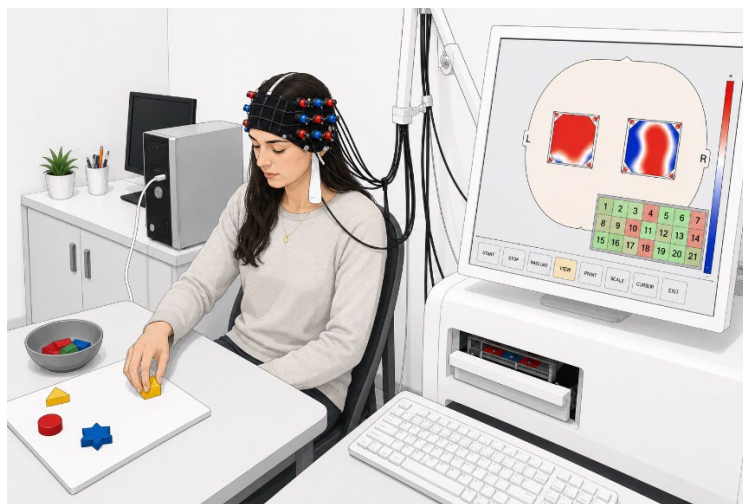
Figure 2.1: Illustration of an fNIRS system setup showing the optode cap, data acquisition unit, and real-time brain activation display.
